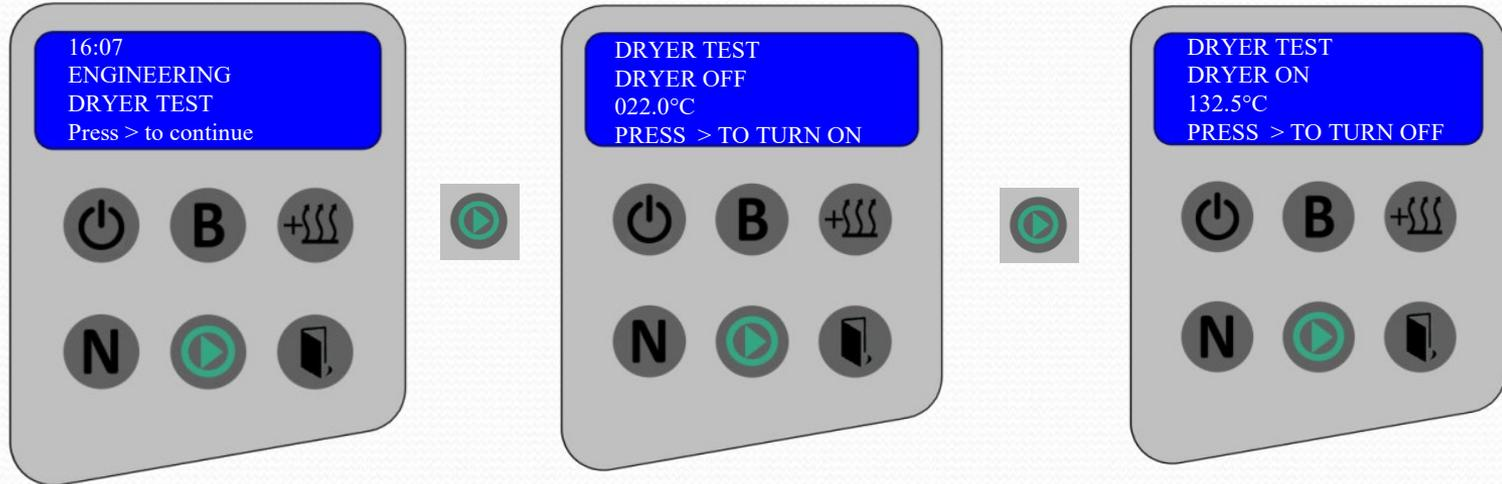
Pressing the Start Switch turns the drying heater on. [The temperature shown on line 3 should climb eventually controlling at 150°C.]
