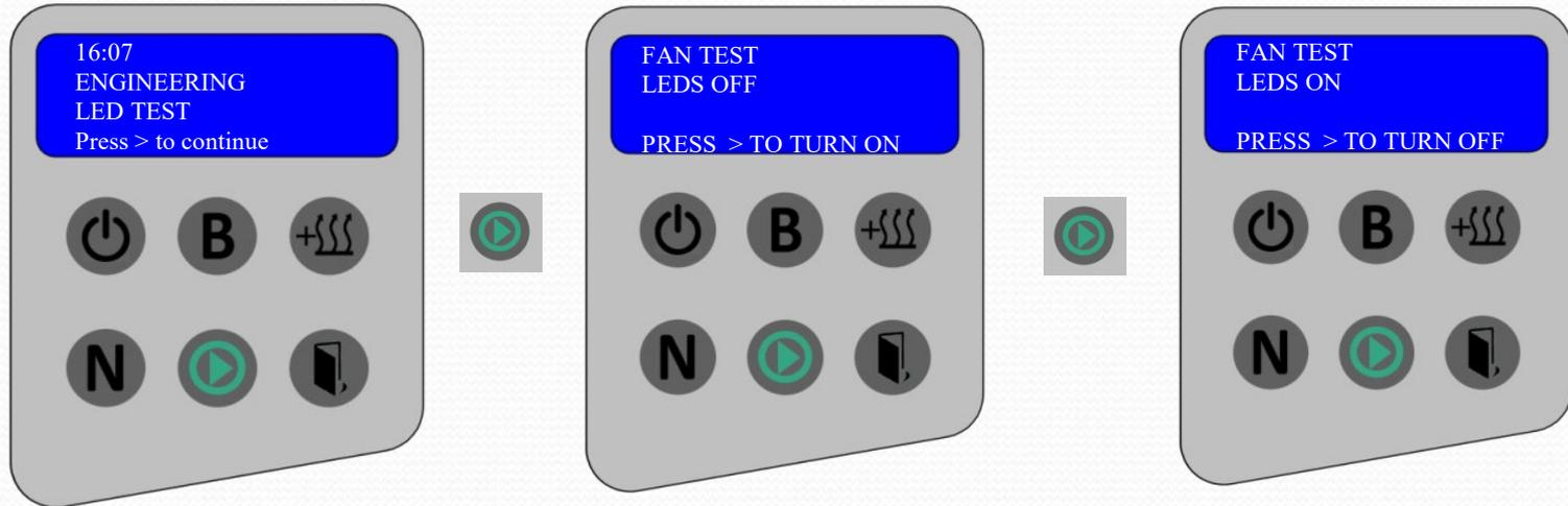
Pressing the Start Switch starts the LED colour sequence.
