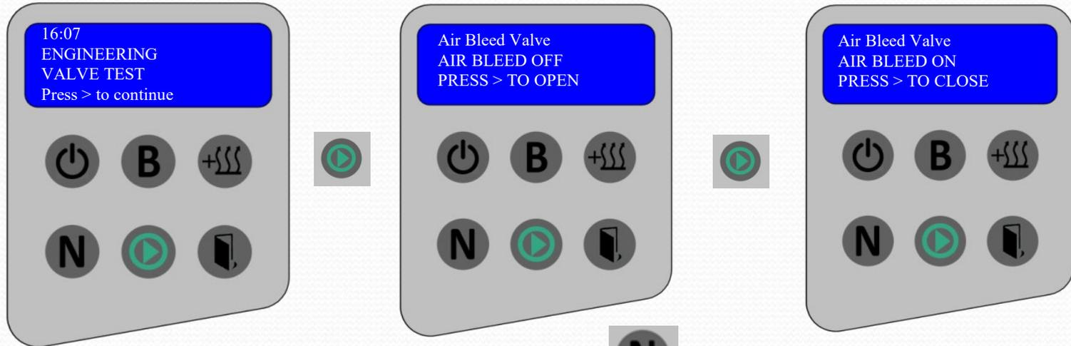
Pressing the cycle start button opens or closes the stated valve. Pressing **N** allows you to change the valve. When you change the valve the default is always Valve OFF.
